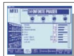
■ MFX Edit Window Use this screen to edit the four major parameters of an MFX processor. Simply twist the Fantom-S/-S88's knobs and the changes are reflected onscreen. More detailed parameter editing is also available.
