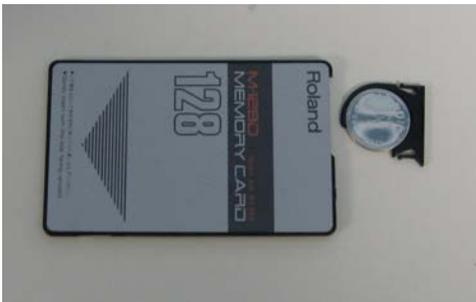
Make a note of which side of the battery is facing up so you can position the new battery correctly.
