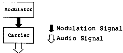
Fig. 2. FM Sound Source Basic Algorithm
