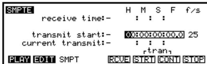
**receive time** This field shows the current time being fed to the SMPTE reader from an external source. It will also detect the frame rate used on the external source and this is displayed underneath the 'f/s' field shown in the top right hand corner of the screen.
