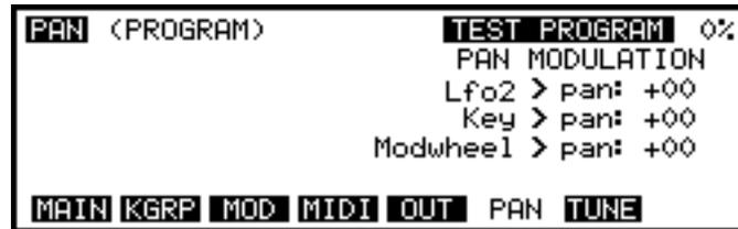
As usual, the program name of the program currently selected for editing is shown here which you may change if you like. As in the OUTPUT page, we have three modulation inputs which can control panning. The defaults for these three control inputs are:
