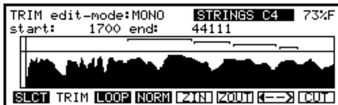
This shows the waveform of the selected sample. You may edit the start and end of the sample accordingly.
