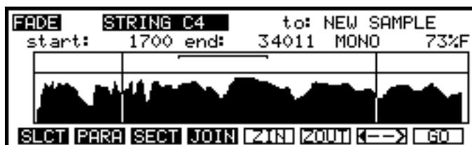
Here we see a string sample and a start and end time has been set (the sample's loop is shown above the waveform display). Pressing **GO** will give you the usual prompts if you have not created a new sample to copy to. If you agree to overwriting the original sample or have created a new one, after a few seconds you will receive a display not unlike this one:
