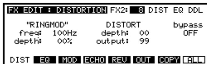
Here, you can add ring modulation and distortion to a sound.
