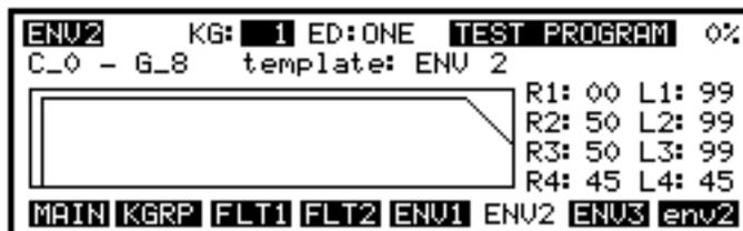
This is a 4-stage envelope generator with 4 rates going to 4 levels. Basically, Rate 1 goes to Level 1, Rate 2 to Level 2, Rate 3 to Level 3 (which is also the sustain) and Rate 4 goes to Level 4. Again you have a choice of templates from which to choose a variety of preset envelopes (probably a bit more necessary in light of the added complication of a multi-stage envelope) and this works on the same principle as ENV1's templates except that there are more of them.
