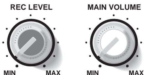
Input level for sampling is regulated using the RECORD LEVEL control and the S3200XL's overall output level is controlled, not surprisingly, by the MAIN VOLUME control. This also governs the level of the sound appearing at the HEADPHONE OUTPUT.
