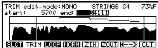
As with the `start:` field, you may move the cursor around the numeric field using the `+/<` and `-/>` keys found on the numeric keypad. Running across the top of the waveform display you will see up to four horizontal lines which show you where you have set your loop point(s). Up to four may be shown simultaneously - the top one is LOOP 1, the second one down is LOOP 2, the next one down LOOP3 and the bottom one is LOOP 4. I.e:
