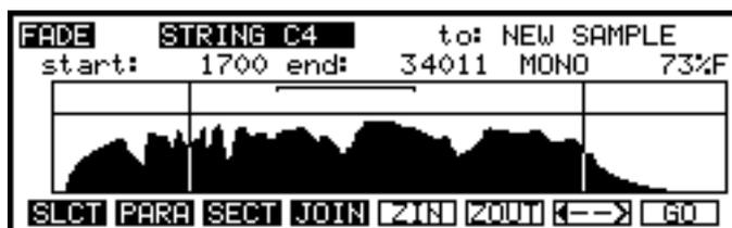
Here, you can see the sample has fades which lead up to the points set by the start and end positions set above. You may play the sample from your keyboard or the ENT/PLAY key.
