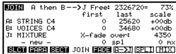
The samples to be joined together are known here as A and B, and the resulting JOINed sample is called J. Though A and B can be the same sample, the resulting (J) sample cannot be the same as either A or B. Press the NAME key to enter a new sample name for the sample J. Existing samples can be overwritten and therefore can be used for J.
