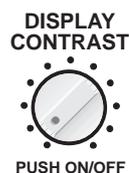
You may adjust the viewing angle for the screen using the DISPLAY CONTRAST control.
