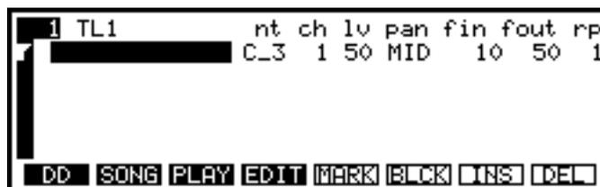
You may now select a take using the data control (or the +/< or -/> keys found on the numeric keypad). Having done that, the selected take's parameters will be loaded into the step and so the note, level, pan and other fields may change if the raw takes parameters are different from those set as the default shown above. You may change these as necessary. Once you have assigned your first take, you should receive a screen something like this:
