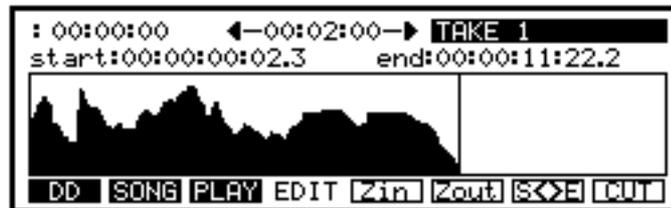
When you enter this page, you see a graphic representation of the take's waveform and you may move the start and end points around freely. The start and end points are shown both as time values in the start: and end: fields respectively and are also shown as flashing vertical lines in the waveform display. You may zoom in or out on a waveform for greater editing accuracy. The fields are as follows:
