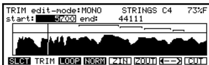
You will see a vertical line indicating the position of the start point. This is adjusted using the DATA control.
